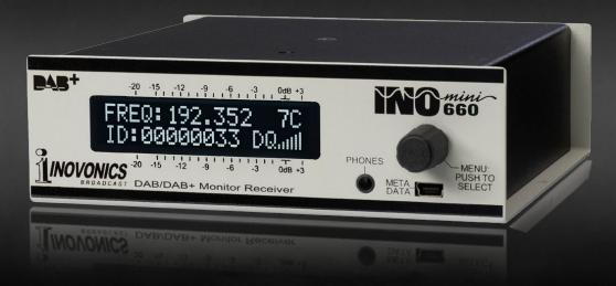
The INOmini 660 is an off-air monitoring receiver for EBU-specified DAB and DAB+ digital radio broadcast transmissions. It provides high-quality confidence monitoring with both balanced analog and AES-digital program line outputs.
